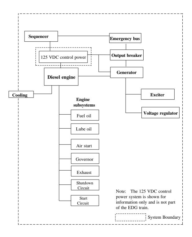
Figure 1. Simplified EDG train schematic.
