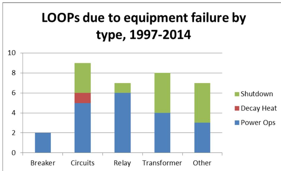
Figure 8. LOOP equipment failures by type.
