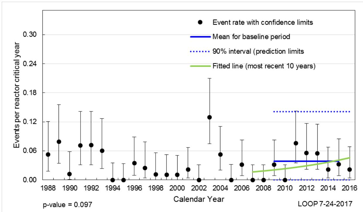
Figure 1. Loss of offsite power initiating event frequency.
