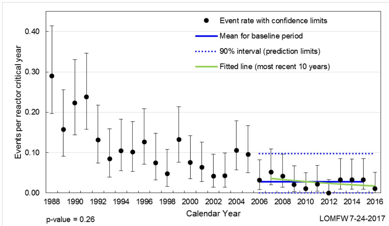
Figure 6. Loss of main feedwater initiating event frequency.
