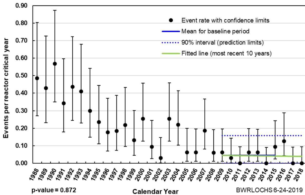
Figure 10. BWR loss of condenser heat sink initiating event frequency.
