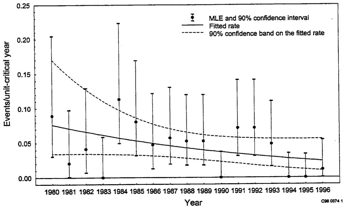
**Figure 3-1.** Frequency of plant-centered LOSP sustained initiating events during operation. When the extra-Poisson scatter is accounted for, the trend is not statistically significant (p-value = 0.11).
