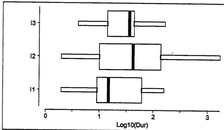
**Figure B-23.**  $\text{Log}_{10}(\text{recovery time})$ , for plant-centered shutdown events with recovery time  $\geq 2$  minutes, plotted by design group. The differences are not statistically significant ( $p\text{-value} = 0.37$ ). The difference between groups I1 and I3 is also not statistically significant ( $p\text{-value} = 0.35$ ).
