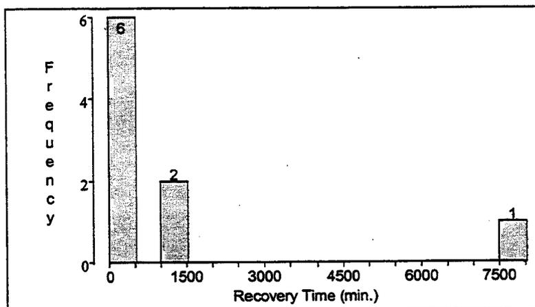
**Figure 3-6.** Histogram of recovery times (minutes) for sustained severe-weather LOSP events. For any event, the recovery times have been averaged for multiple units at a site, and regarded as a single time.
