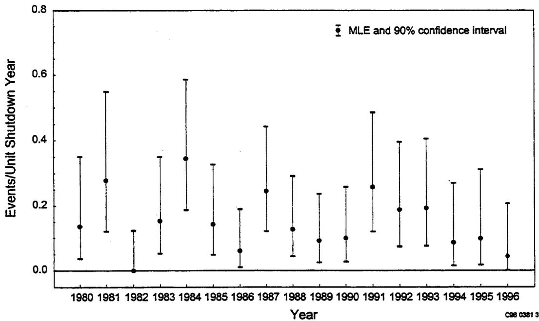
**Figure B-6.** Frequency of plant-centered LOSP sustained events during shutdown. No trend is fitted, because it is not close to statistically significant. Between-unit variation is present, but the confidence intervals for each year ignore this.
