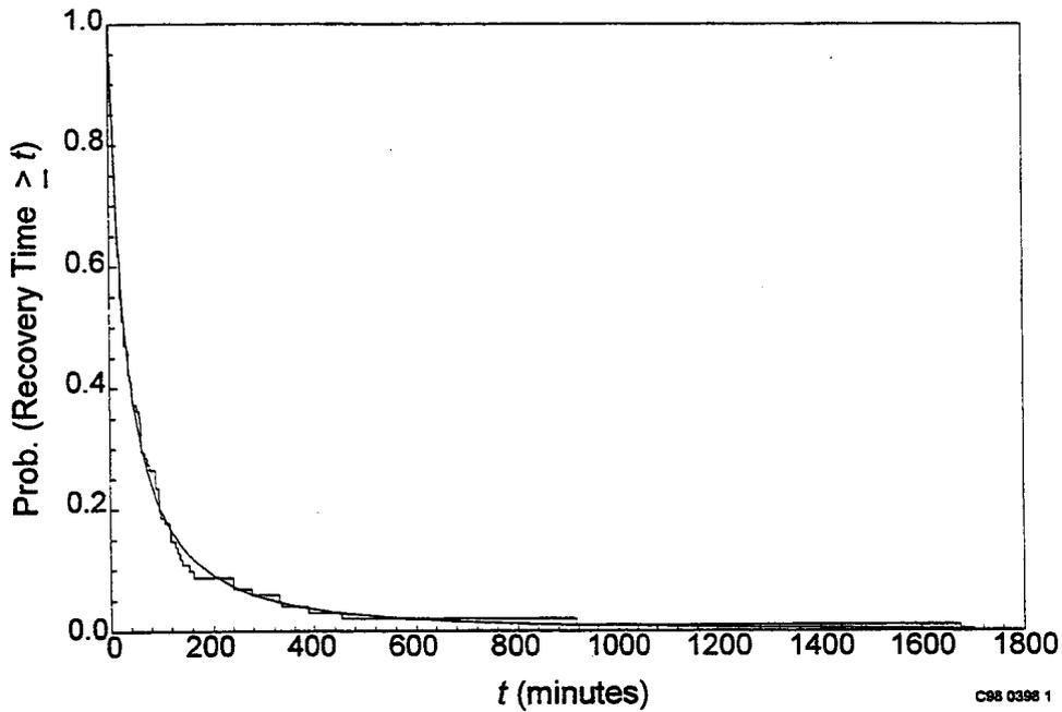
**Figure 3-4.** Recovery curves for recovery time (minutes) of plant-centered sustained trip and shutdown events, empirical and fitted lognormal.
