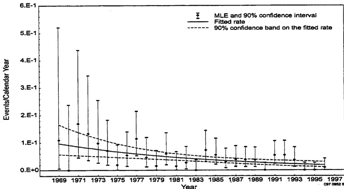
**Figure 3-7.** Frequency of plant-centered LOSP initiating events per unit year. The trend is statistically significant.
