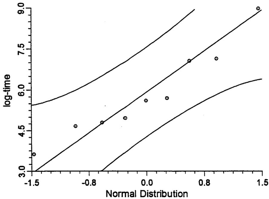
**Figure B-17.** Reported values of  $\ln(\text{recovery time})$  vs. normal quantiles, for severe-weather sustained events. The band represents 95% confidence intervals (in the vertical direction) for the expected values of the ordered observations.
