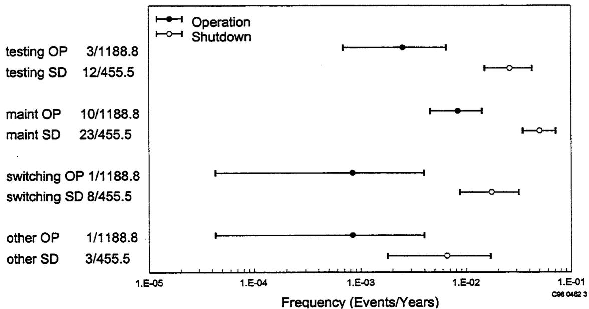
Figure 4-8. Frequencies of human error types, during operation and shutdown. Maximum likelihood estimates and 90% intervals are plotted.
