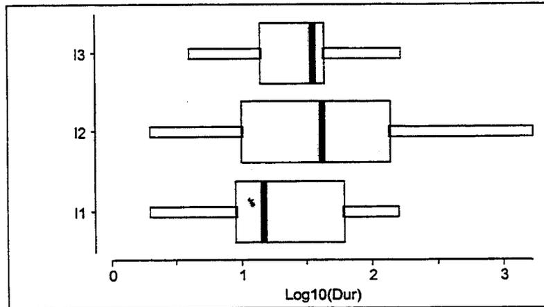
**Figure 3-11.**  $\text{Log}_{10}(\text{recovery time})$ , for plant-centered shutdown events with recovery time  $\geq 2$  minutes, plotted by design group. The differences are not statistically significant ( $p\text{-value} = 0.37$ ). The difference between groups I1 and I3 is also not statistically significant ( $p\text{-value} = 0.35$ ).
