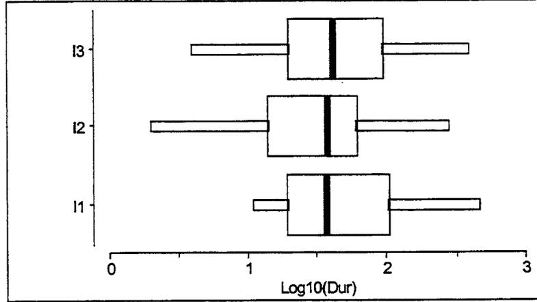
**Figure 3-10.**  $\text{Log}_{10}(\text{recovery time})$ , for plant-centered trip events with recovery time  $\geq 2$  minutes, plotted by design group. The differences are not statistically significant ( $p\text{-value} = 0.39$ ).
