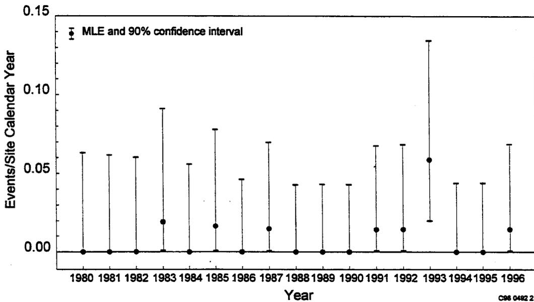
**Figure B-8.** Frequency of severe-weather LOSP sustained events. No trend is fitted, because it is not statistically significant. The large frequency in 1993 is the result of a single storm affecting several power plant sites. The confidence intervals for each year ignore between-site variation.
