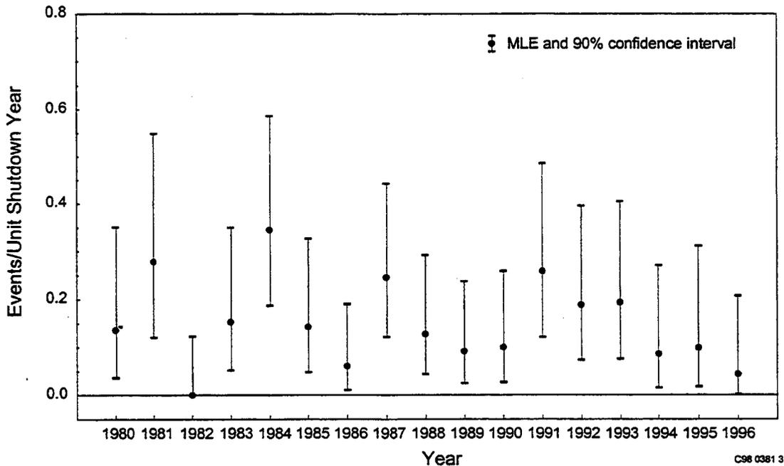
**Figure 3-2.** Frequency of plant-centered LOSP sustained events during shutdown. No trend is fitted, because it is not close to statistically significant. The confidence intervals for each year do not account for between-unit variation.
