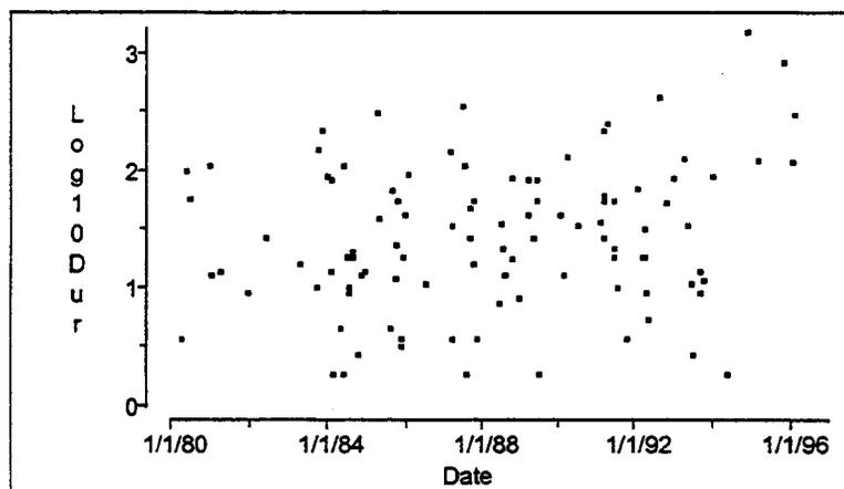
**Figure B-13.** For sustained plant-centered events, plot of  $\log_{10}(\text{recovery time})$  against event date. A slight upward trend is statistically significant ( $p\text{-value} = 0.03$ ), but is not modeled for reasons discussed in the text.
