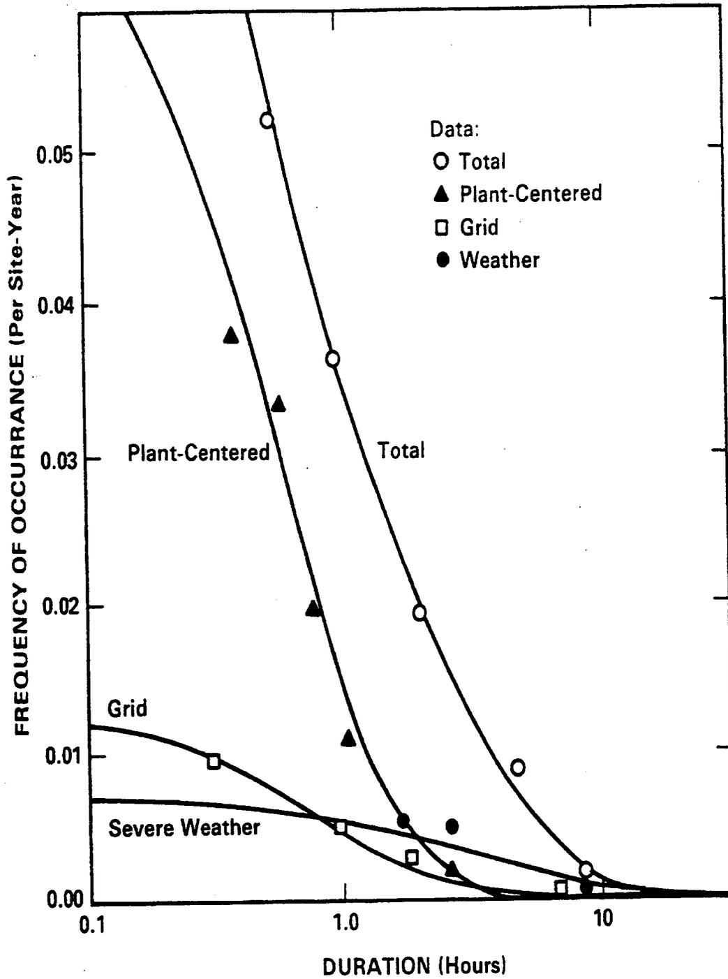
Figure 3-8. Complementary cumulative frequency curves, from NUREG-1032. Height of curve equals frequency of exceeding the time on the horizontal axis.
