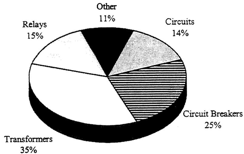
**Figure 4-3.** LOSEP events caused by equipment failures, by equipment type.
