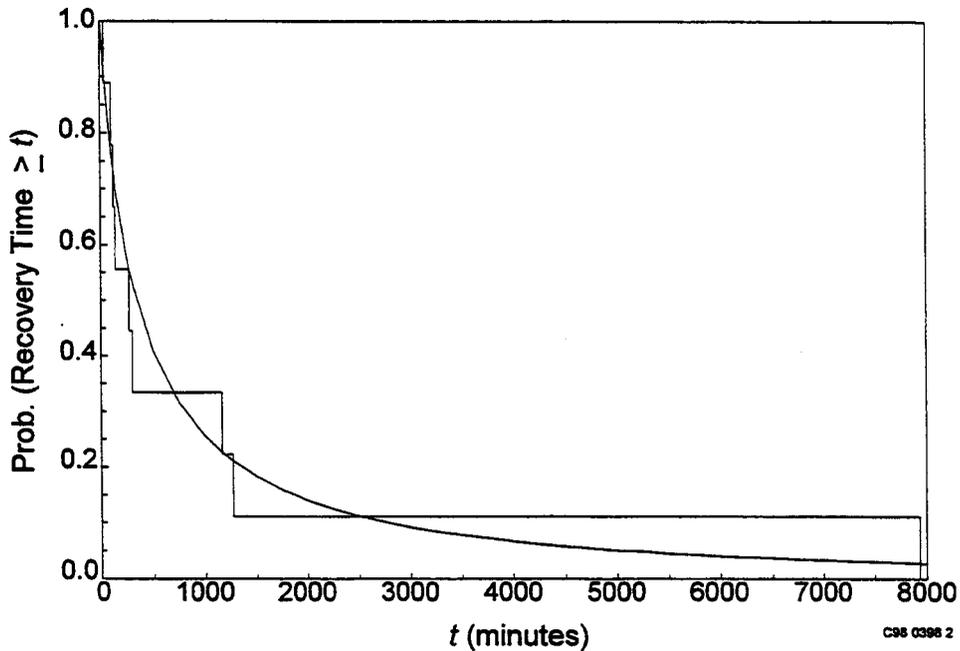
**Figure B-19.** Recovery curve for severe-weather recovery times, empirical and fitted lognormal. This is based on sustained trip and shutdown events.
