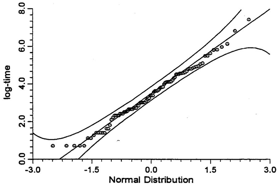
**Figure B-16.** Reported values of  $\ln(\text{recovery time})$  vs. normal quantiles, for plant-centered sustained trip and shutdown events. The band represents 95% confidence intervals (in the vertical direction) for the expected values of the ordered observations.
