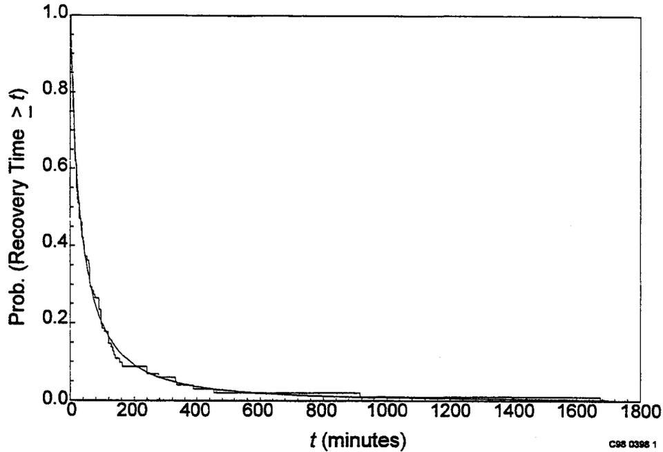
**Figure B-18.** Recovery curve for plant-centered recovery times, empirical and fitted lognormal. This is based on sustained trip and shutdown events.
