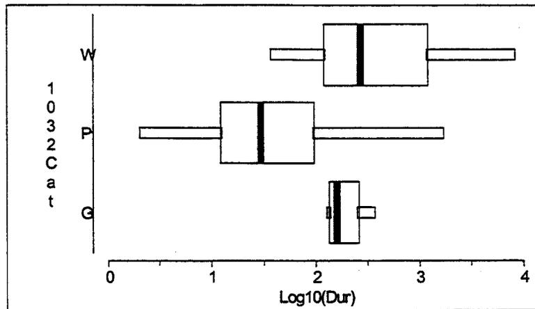
**Figure B-12.** Logarithms of sustained recovery times for the three 1032-categories of events whose recoveries are analyzed separately. The difference between severe-weather and plant-centered times is statistically extremely significant.
