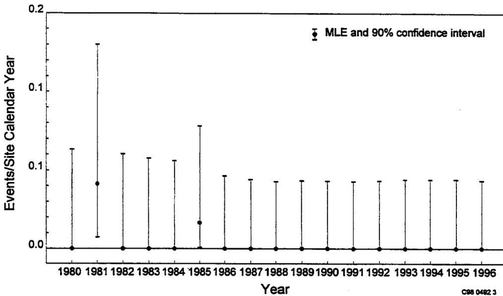
**Figure B-7.** Frequency of grid-related LOSP sustained events, both initiating events and shutdown events. No trend is fitted, because it is apparently not significant. However, the sparsity of data and possible dependence of events complicate significance calculations.
