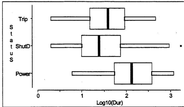
**Figure B-9.** Logarithms of sustained recovery times, for three classes of plant-centered events. The power-operation recovery times are longer than each of the other groups of recovery times, to a statistically significant degree. The difference between trip and shutdown times is not statistically significant (p-val. = 0.3).
