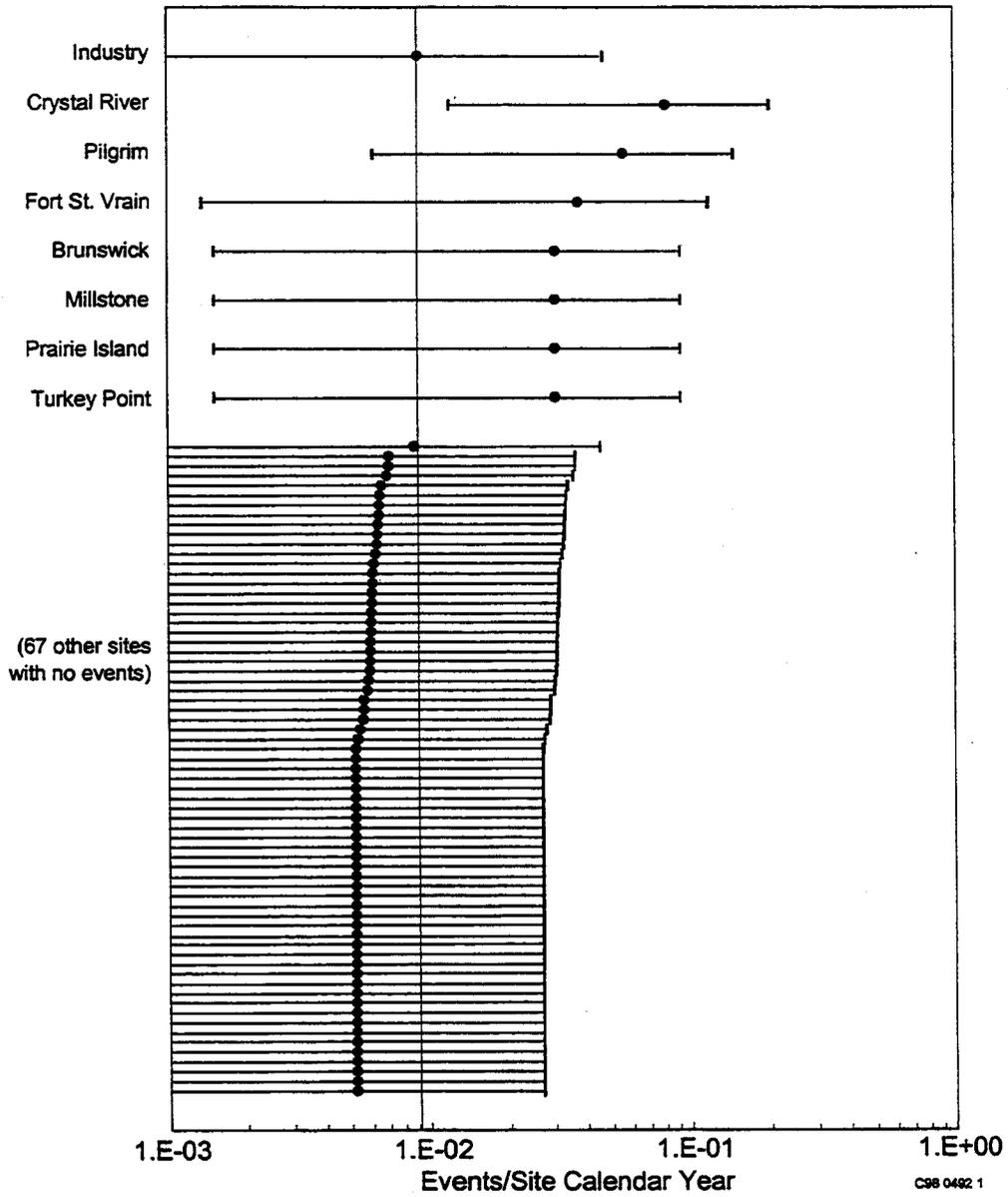
**Figure B-4.** Frequency of severe-weather LOSP sustained events. The empirical Bayes estimate and 90% uncertainty interval are shown for each power plant unit. The left ends of many intervals extend far to the left of the visible portion of the figure, and are not meaningful.
