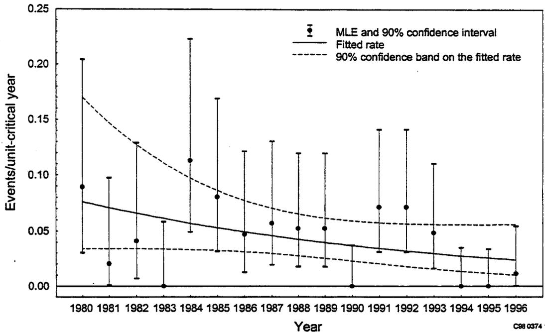
**Figure B-5.** Frequency of plant-centered LOSP sustained initiating events during operation. When the extra-Poisson scatter is accounted for, the trend is not statistically significant (p-value = 0.11).
