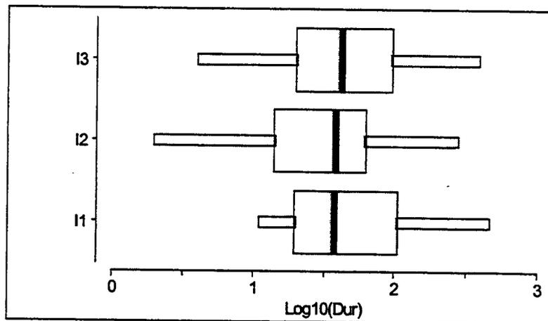
**Figure B-22.**  $\text{Log}_{10}(\text{recovery time})$ , for plant-centered trip events with recovery time  $\geq 2$  minutes, plotted by design group. The differences are not statistically significant ( $p\text{-value} = 0.39$ ).
