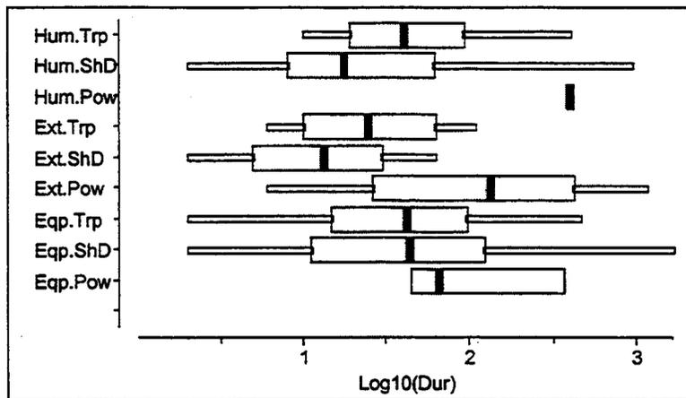
**Figure B-10.** Logarithms of sustained recovery times of plant-centered events, for combinations of event cause and unit condition. The differences are not statistically significant, although when combined as in Figure B-9 some differences are statistically significant.
