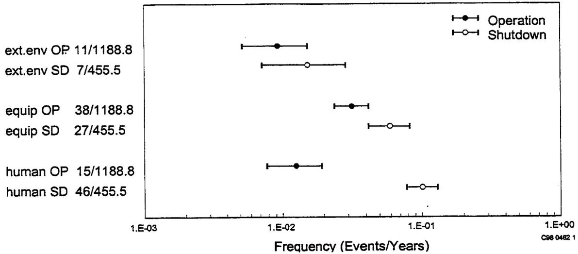
**Figure 4-2.** Frequencies of major causes of plant-centered events. The number of events per reactor critical year or events per reactor shutdown year is printed on the left. Maximum likelihood estimates and 90% confidence intervals are plotted.
