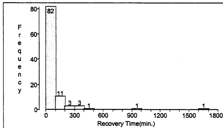
**Figure 3-3.** Histogram showing recovery times (minutes) for plant-centered trip and shutdown events with recovery times  $\geq 2$  minutes. This plot does not show 11 momentary events and 9 events with unknown recovery times. For any event at multiple units, only one site-average recovery time is counted.
