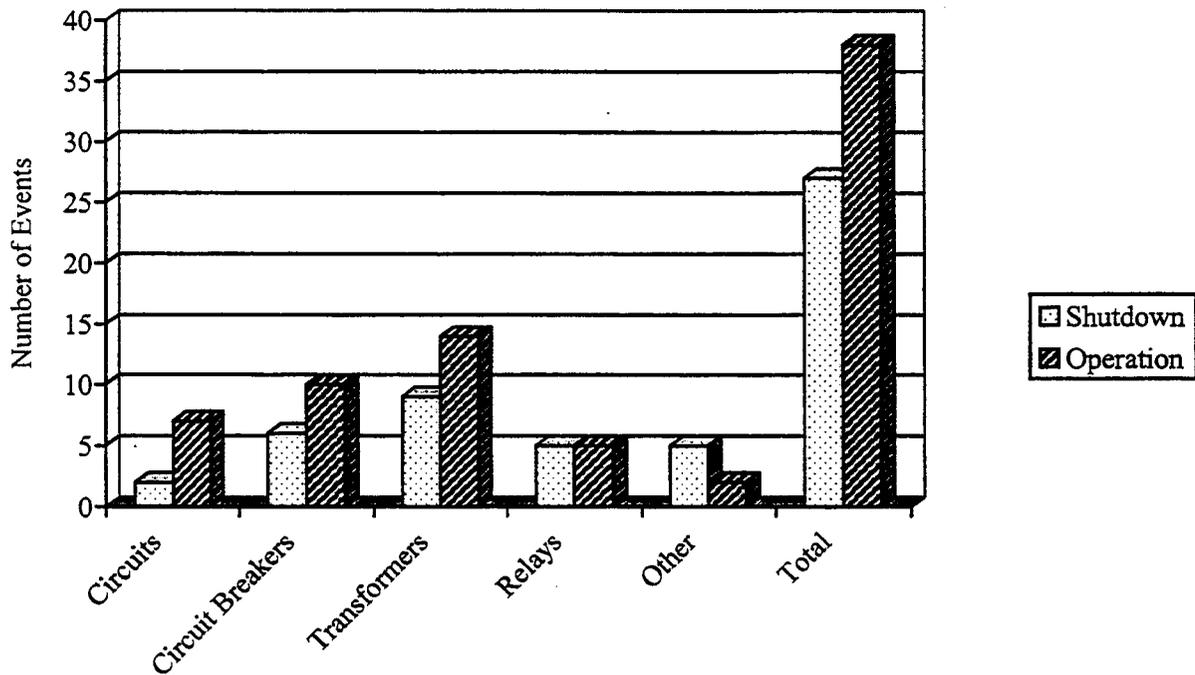
Figure 4-4. Number of LOSP events caused by equipment failures, by equipment type and unit status.
