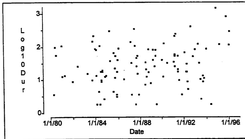
**Figure 3-5.** For sustained plant-centered events, plot of  $\log_{10}(\text{recovery time})$  against event date. A slight upward trend is statistically significant ( $p\text{-value} = 0.03$ ), but is highly dependent on the two points in the upper right, as discussed in the text. Therefore no trend is modeled.
