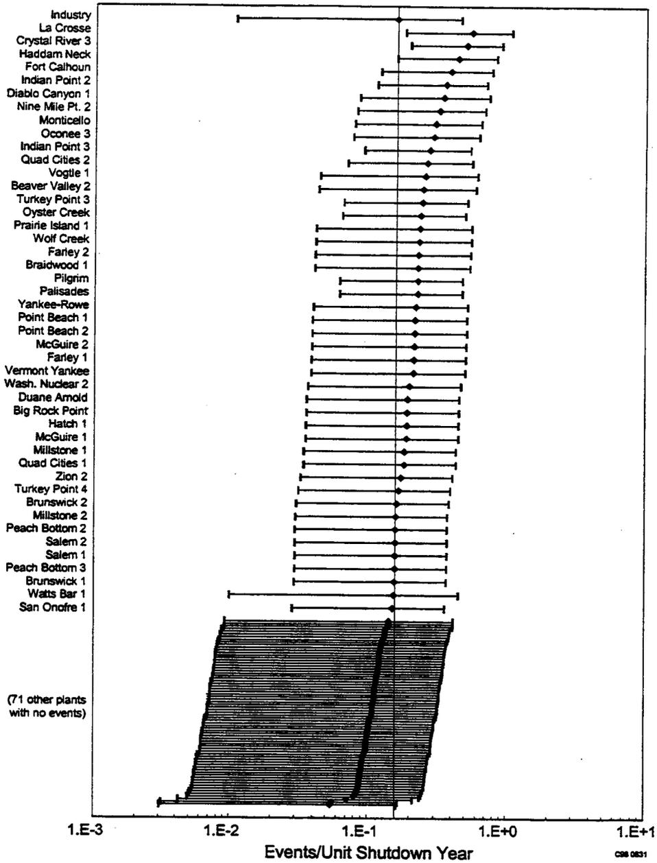
Figure B-3. Frequency of plant-centered LOSP sustained events during shutdown. The empirical Bayes estimate and 90% uncertainty interval are shown for each unit.
