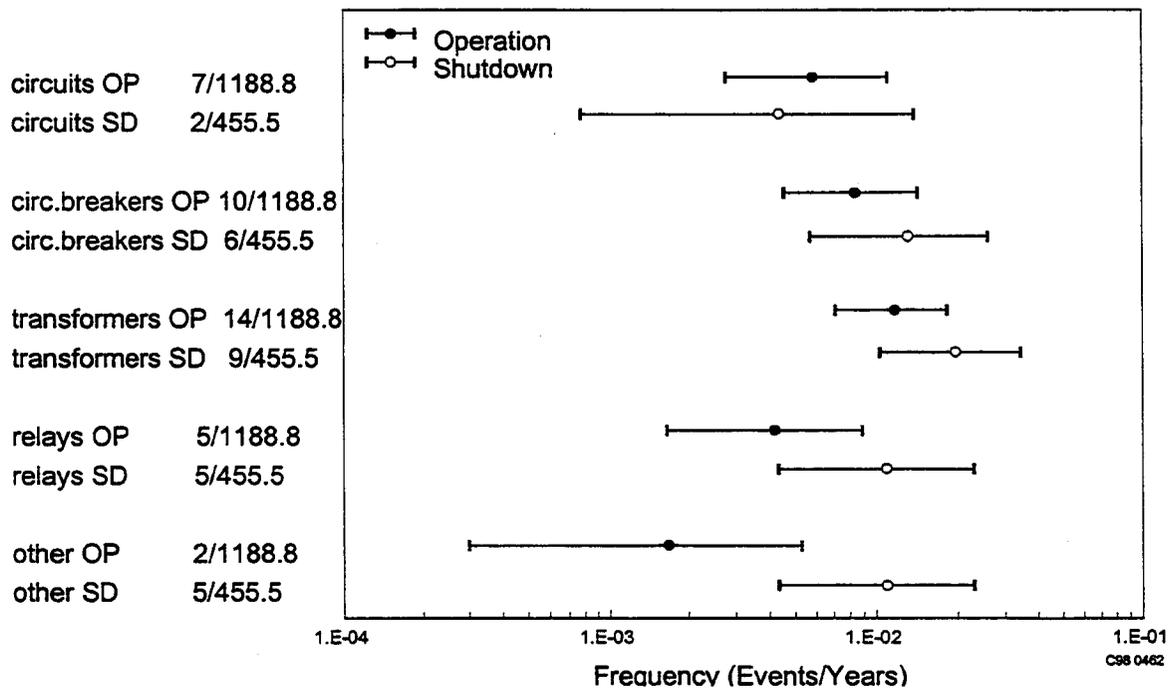
Figure 4-5. Frequencies of equipment failure types, during operation and shutdown. Maximum likelihood estimates and 90% intervals are plotted.
