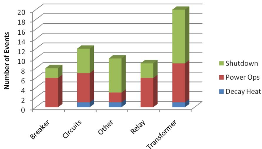
Figure 12. LOOP due to equipment failure by cause, 1986–2010.
