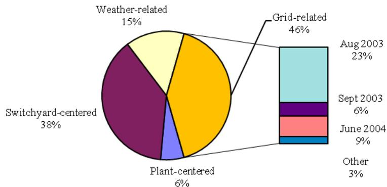
Figure 1. Distribution LOOP categories (per plant unit) during critical operation (1997 to 2010).
