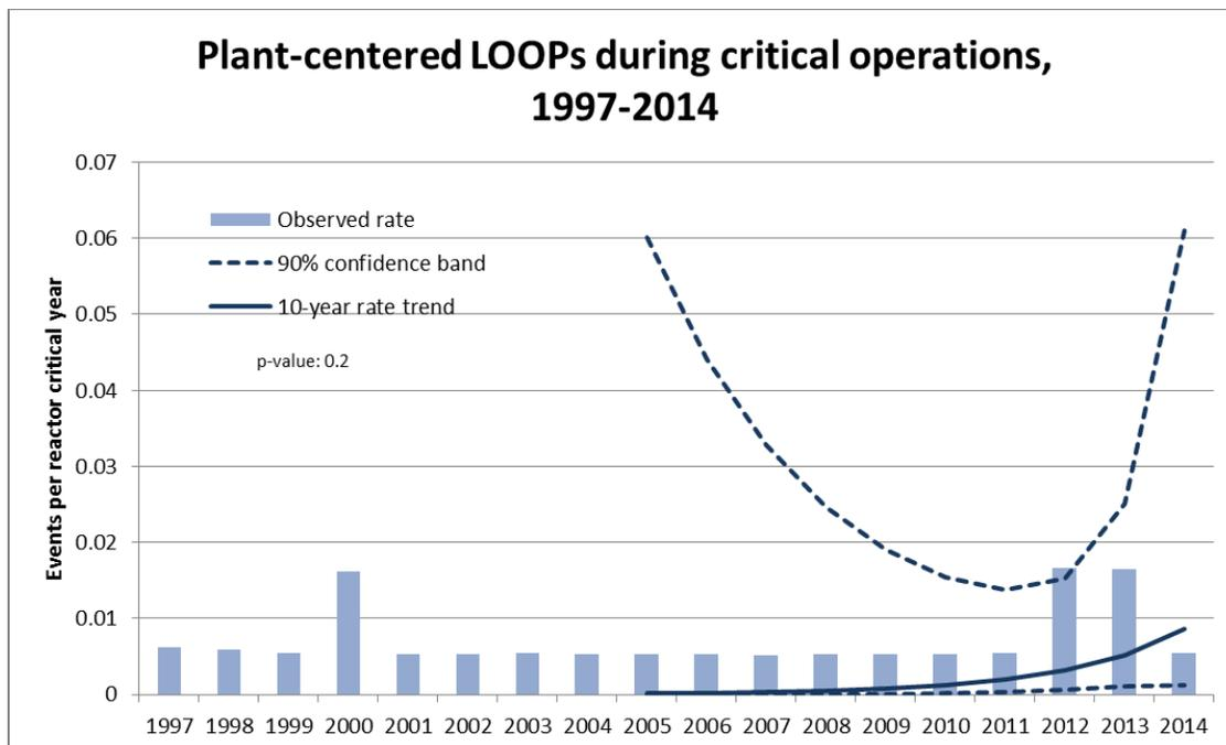
Figure 3. 10-year trend, plant-centered LOOPs during critical operation.
