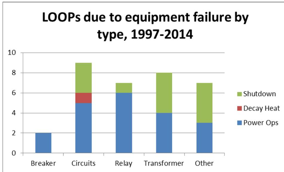
Figure 8. LOOP equipment failures by type.
