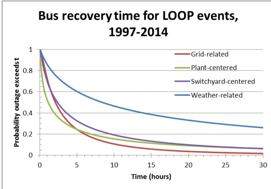
Figure 6. Fitted recovery time distributions.
