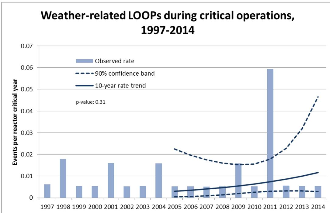
Figure 5. 10-year trend, weather-related LOOPs during critical operation.
