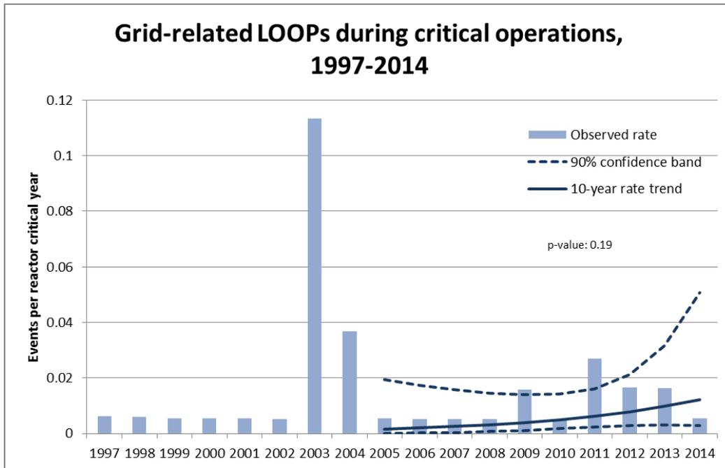
Figure 2. 10-year trend, grid-related LOOPs during critical operation.
