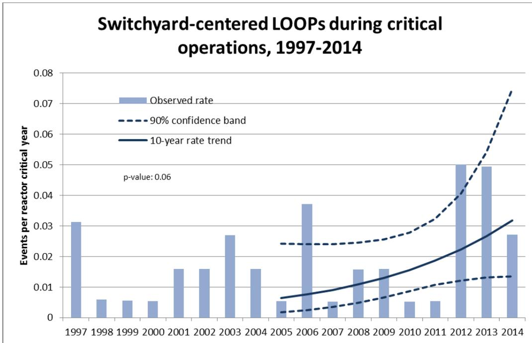
Figure 4. 10-year trend, switchyard-centered LOOPs during critical operation.
