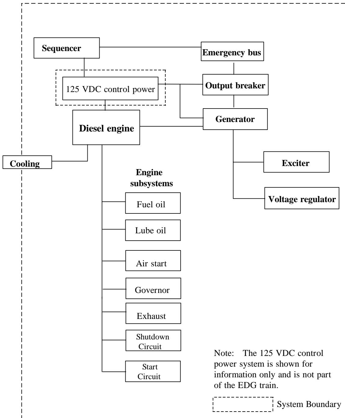
**Figure 1. Simplified EDG train schematic.**
