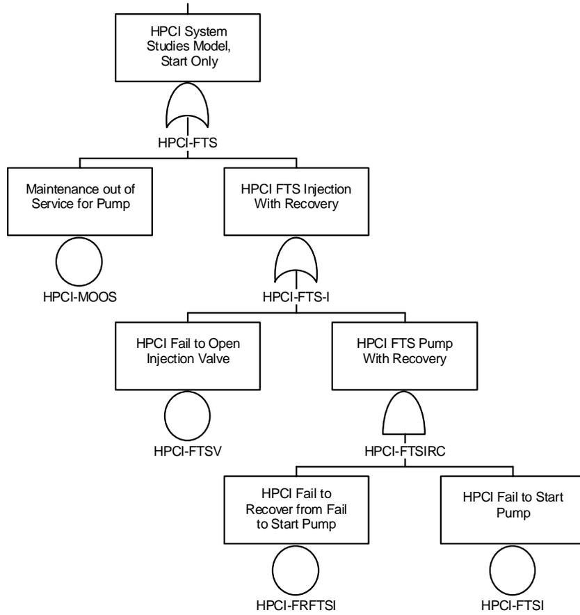
**Figure 2. Unavailability model of HPCI system for a start only mission.**
