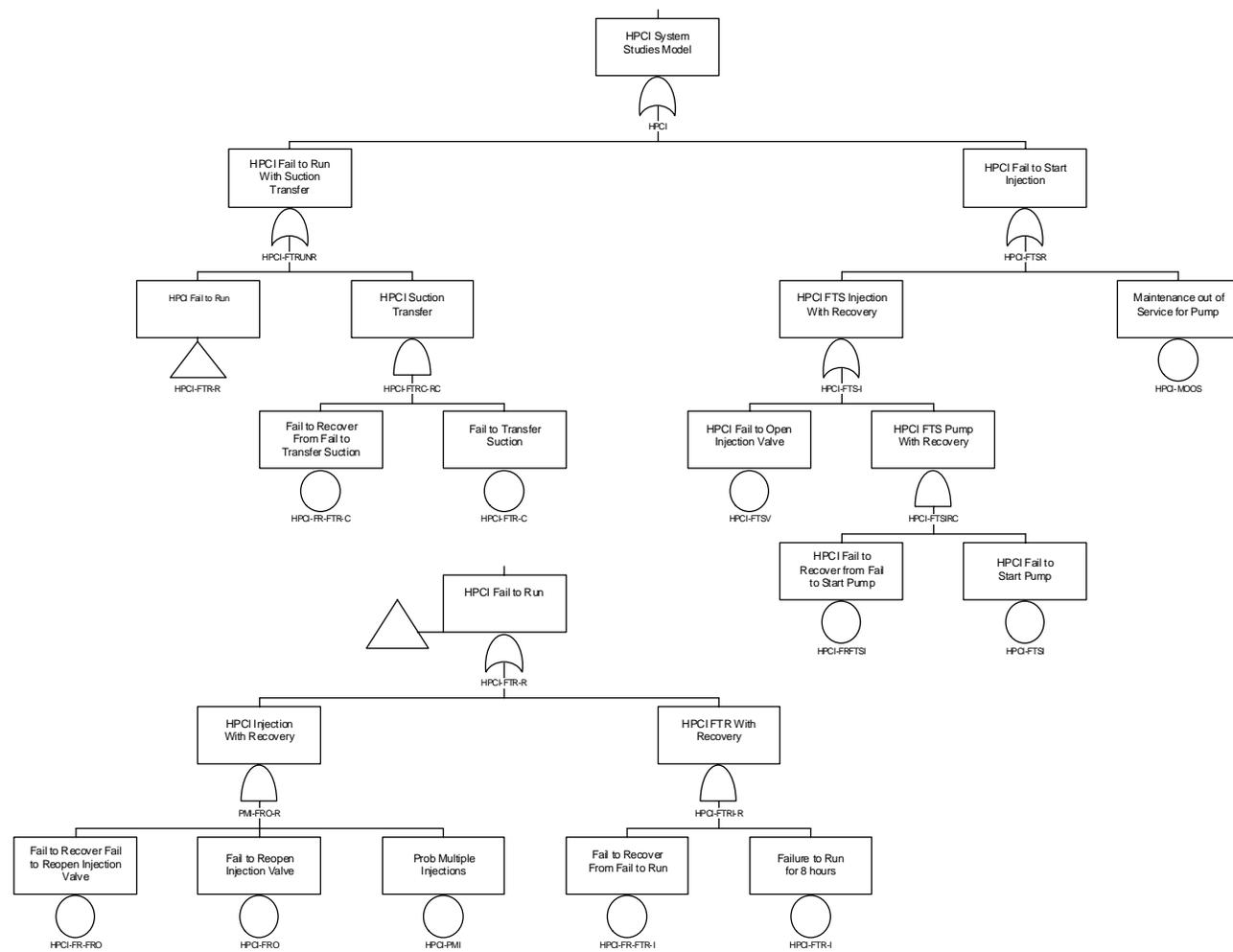
Figure 1. Unreliability model of HPCI operation for an 8-hour mission.
