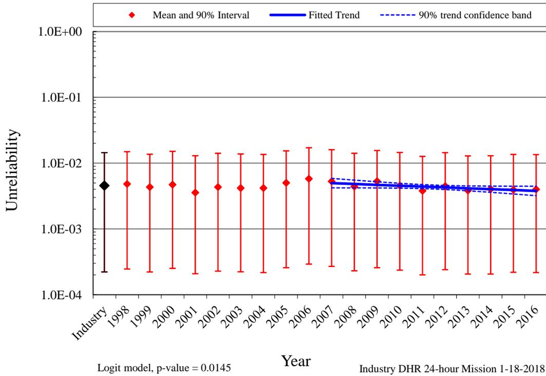
Figure 8. Trend of RHR shutdown cooling mode system unreliability (24-hour model).
