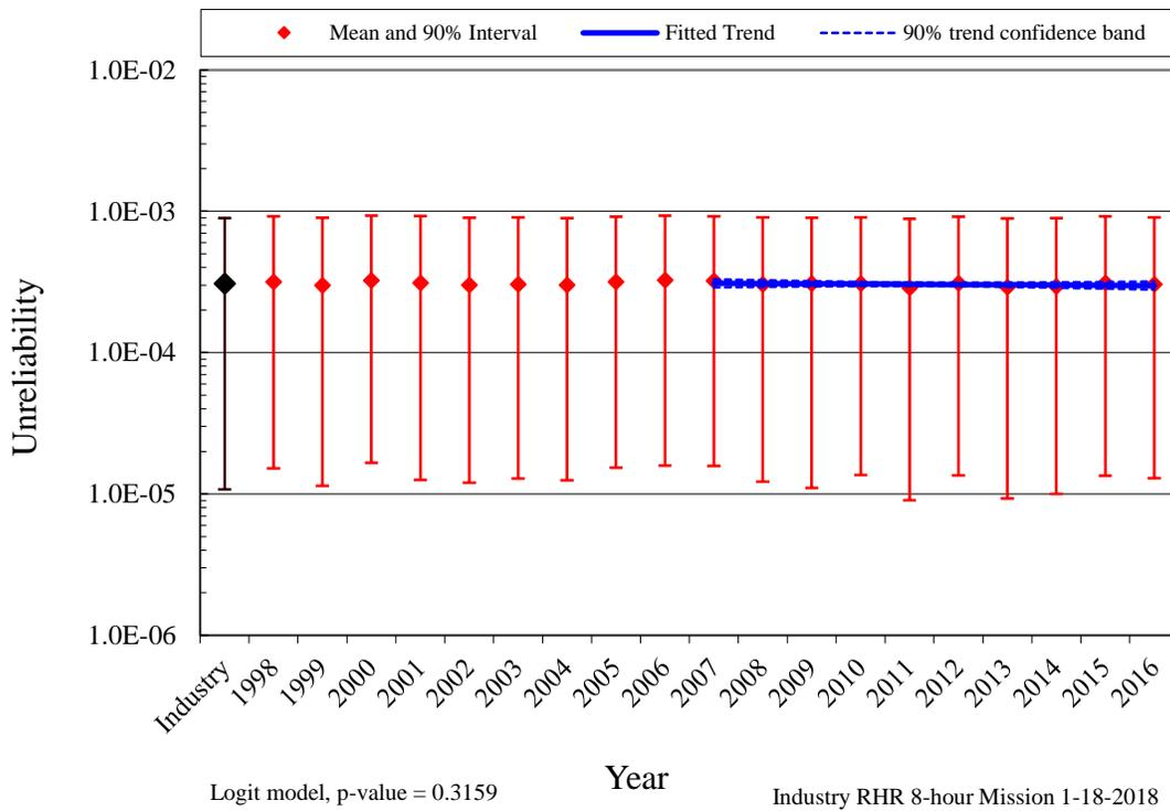
Figure 6. Trend of RHR (injection mode) system unreliability (8-hour model).
