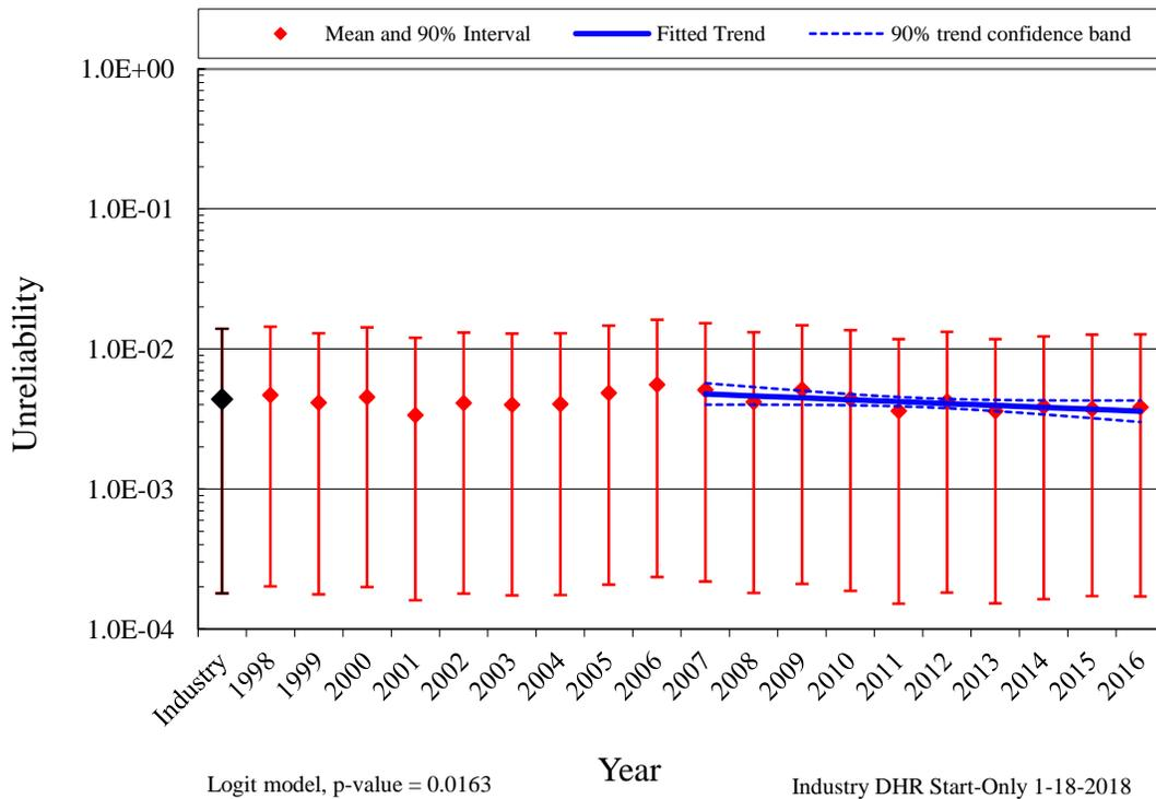
Figure 7. Trend of RHR shutdown cooling mode system unreliability (start-only model).
