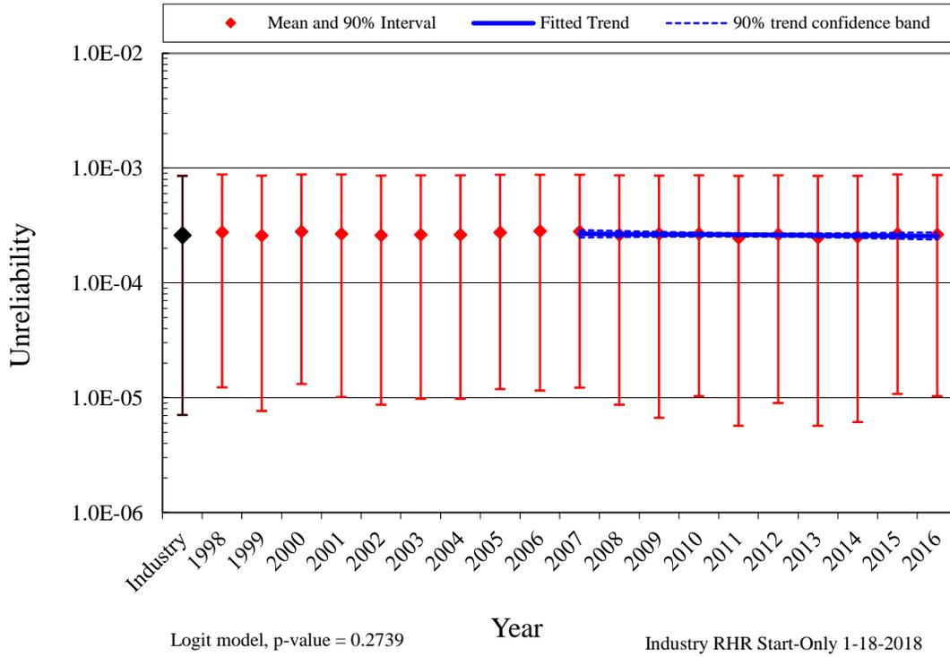
Figure 5. Trend of RHR (injection mode) system unreliability (start-only model).
